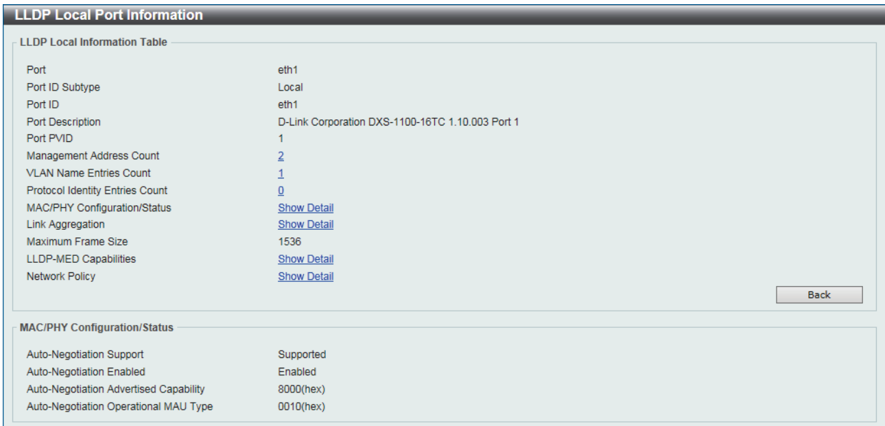
Figure 4.120 – L2 Features > LLDP > LLDP Local Port Information (Show Detail)
