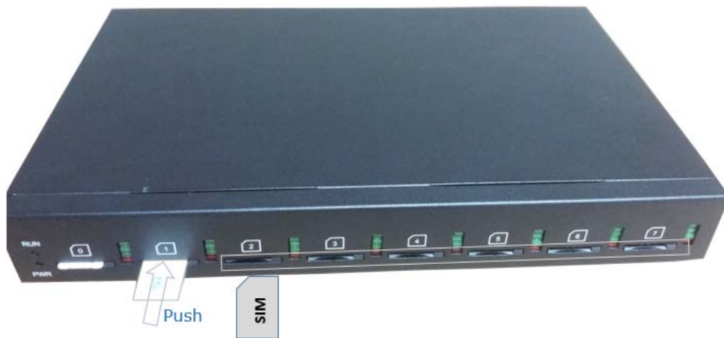
Figure 2-2-1 SIM Card installation
