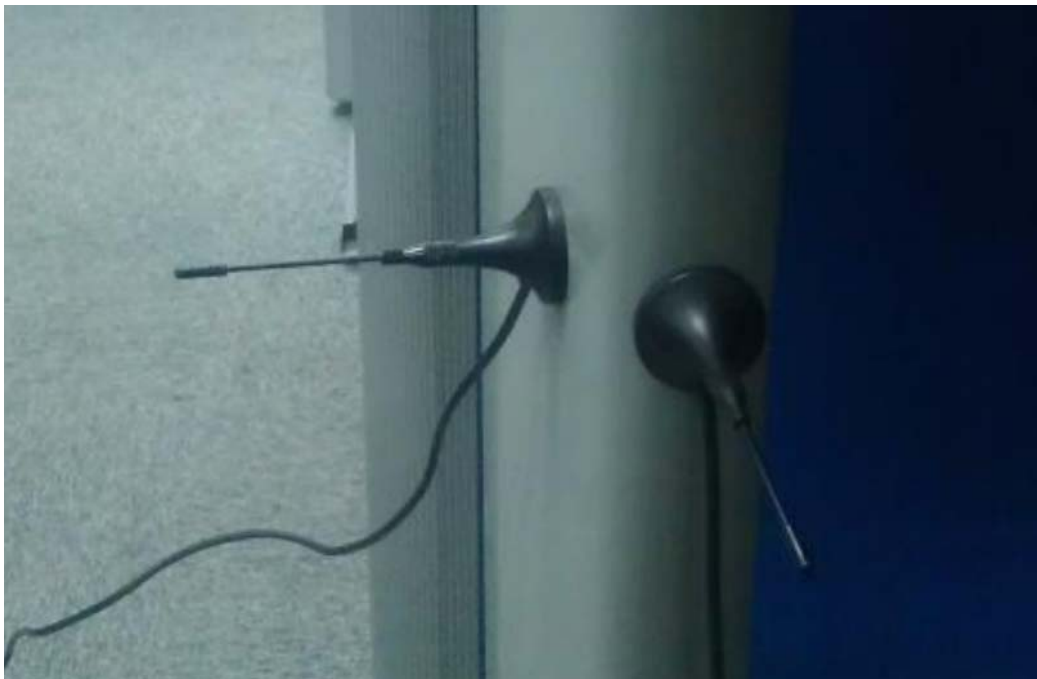
Figure 6.3 Isolation by antenna orthogonal polarization
