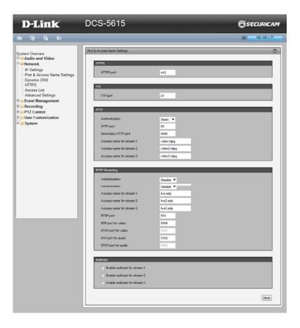
Access name for stream 1 ~ 3: This Network Camera supports multiple streams simultaneously. The access name is used to differentiate the streaming source. If you want to use an RTSP player to access the Network Camera, you have to set the video mode to H.264 / MPEG-4 and use the following RTSP URL command to request transmission of the streaming data.
