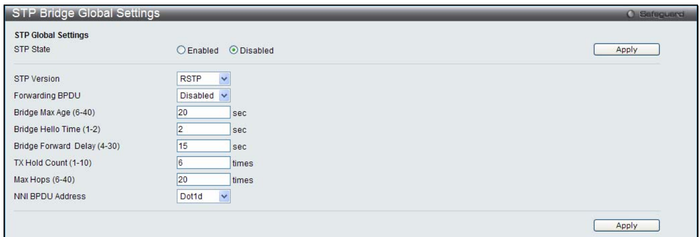
Figure 4-22 STP Bridge Global Settings window
