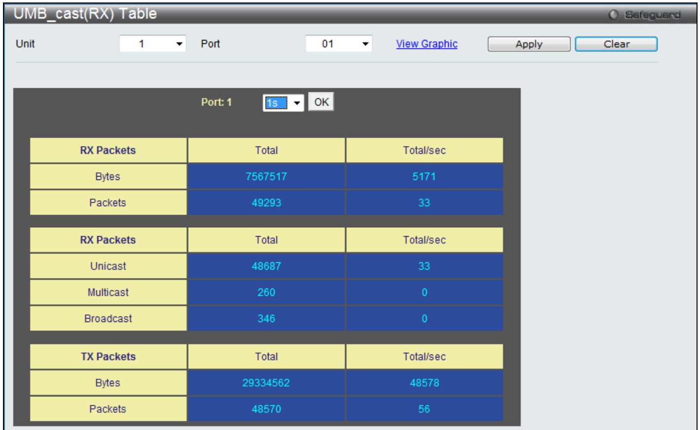
Figure 11-7 RX UMB_cast (RX) Table window (table for Unicast, Multicast, and Broadcast Packets)
