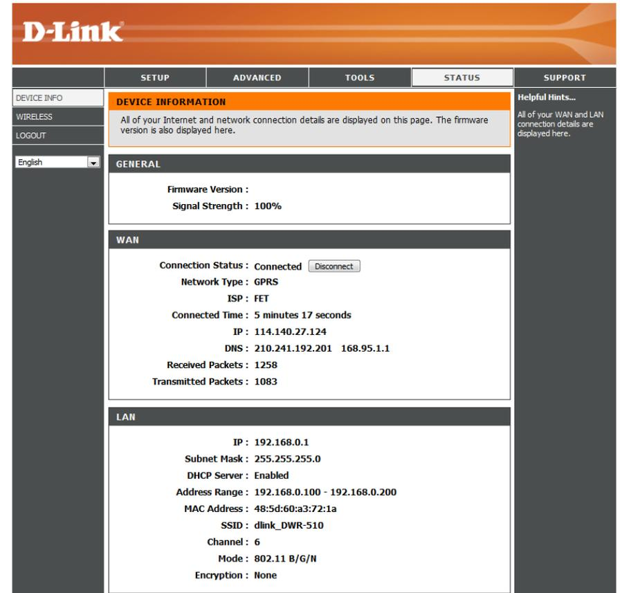
The screenshot shows the D-Link web interface for the DWR-510. The top navigation bar includes tabs for SETUP, ADVANCED, TOOLS, STATUS, and SUPPORT. The main content area is titled "DEVICE INFORMATION" and contains a summary of the page's purpose. Below this, there are three main sections: GENERAL, WAN, and LAN.
