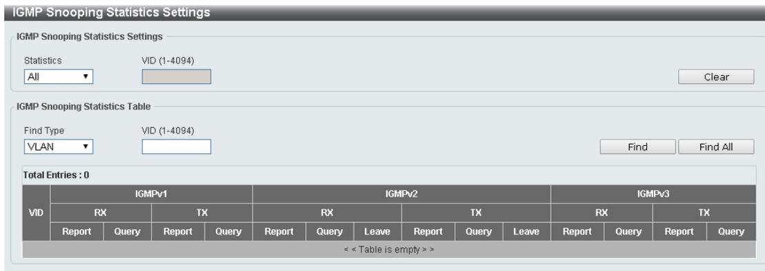
Figure 4.79 – L2 Features > L2 Multicast Control > IGMP Snooping > IGMP Snooping Statistics Settings
