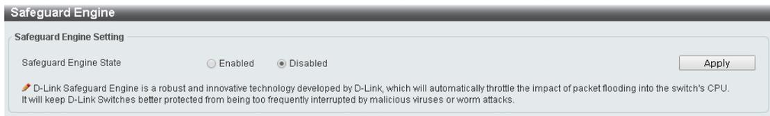
Figure 4.154 – Security > Safeguard Engine
