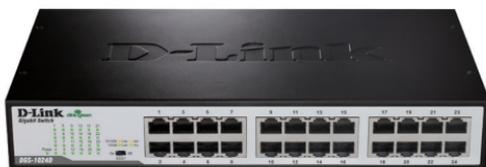
**Link/Act/Speed (1-24)** - This LED indicator light is green when the port is successfully connected to a 1000Mbps device and will blink as data is transmitted or received. This LED indicator light is amber when the port is successfully connected to a 10/100Mbps device and will blink as data is transmitted or received.
