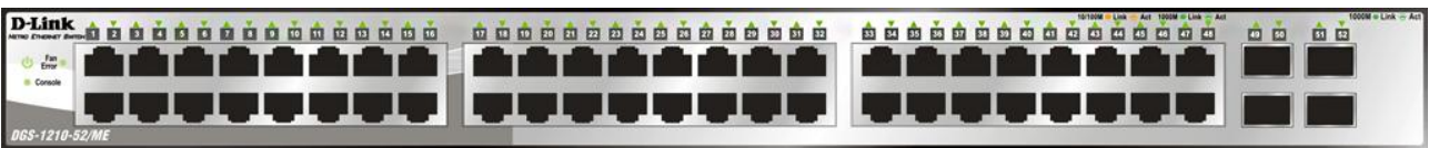
Figure 1.3 – DGS-1210-52/ME SERIES Front Panel
